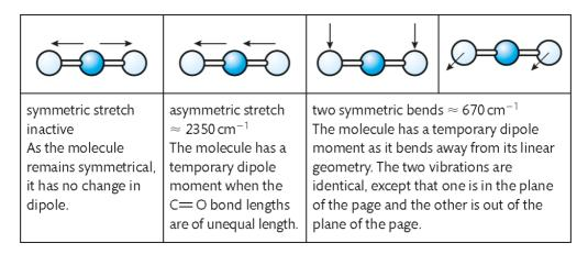
Molecules with several bonds can vibrate in many different ways and with many different frequencies. The complex pattern can be used as a fingerprint to be matched against the recorded spectra of known compounds in a database. A comparison of the spectrum of a sample with that of a pure compound can also be used as a test of purity.
